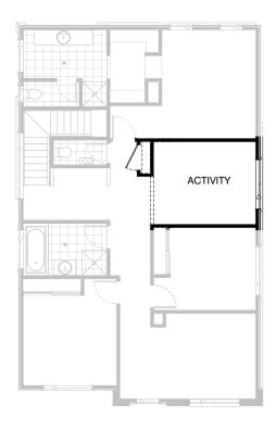
Provide Activity option in lieu of Bed 3 by removing bed 3 hinged door and built-in robe.
