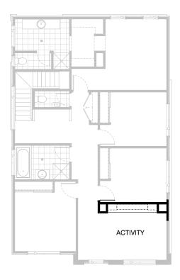
Provide built-in joinery option to Activity room including: 450mm deep 32mm laminate benchtop, 1No. 1000mm TV cupboard drawer unit,
