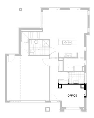
Provide built-in joinery option to Office including: 450mm deep 32mm laminate benchtop, 3No. 800mm TV cupboard drawer units, 3No. 800mm overhead cupboards.
