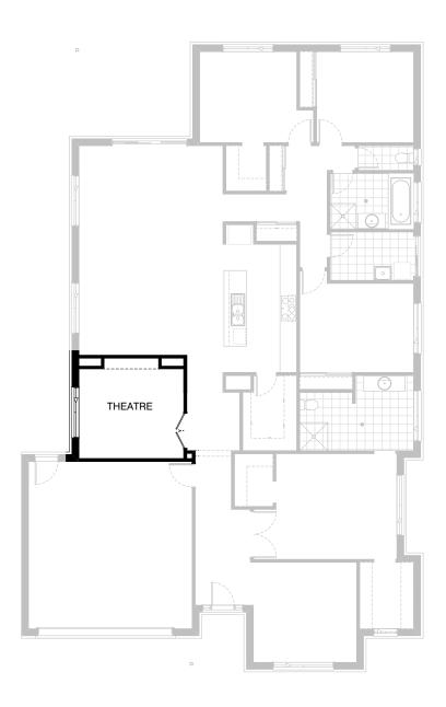
Convert standard Media room into Theatre room including double 2040mm x 620mm flush panel hinged doors, additional plaster lined stud wall and feature wall with plaster columns and bulkhead above and relocate window by 120mm to suit.
