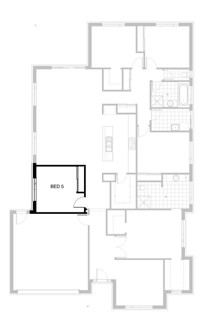
Provide Bed 5 in lieu of Media room with 1no. 820mm flush panel hinged doors and site built plaster lined robe with 1no. hanging rail and shelf with 2no. sliding doors and 1200mm x 1810mm sliding window in lieu of standard 2100mm x 1810mm sliding window.
