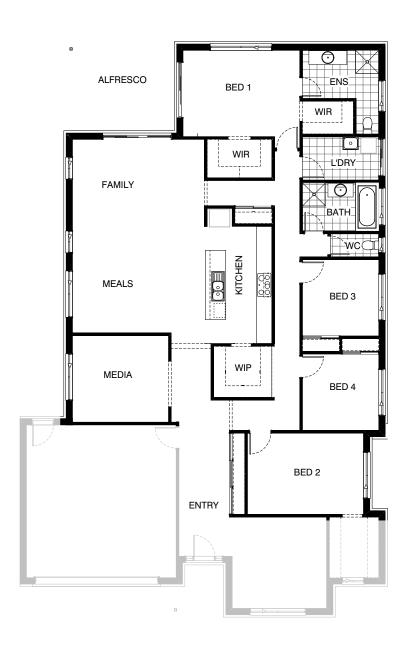
Provide floor plan option with Bed 1 to the rear of the home. Windows replaced and relocated as shown. Option adds ASD2121 sliding door to Bed 1.
