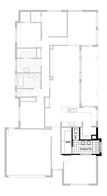
Provide Ensuite upgrade option with rearranged layout, including: 1482mm vanity with double basins, 1770mm x 900mm tiled shower base wih grate drain, enclosed WC with 720mm hinged door. Provide 350mm x 1450mm aluminium frame sliding window with tiled reveals in lieu of standard. Remove Coats cupboard to Passage and reconfigure Walk-in Robe as shown.
